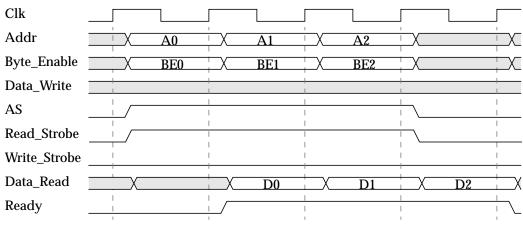
Figure 2-5: LMB Single Cycle Back-to-Back Read Operation
